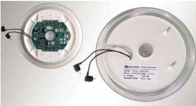
MarkLED® Electronics sealed with sealing compound
