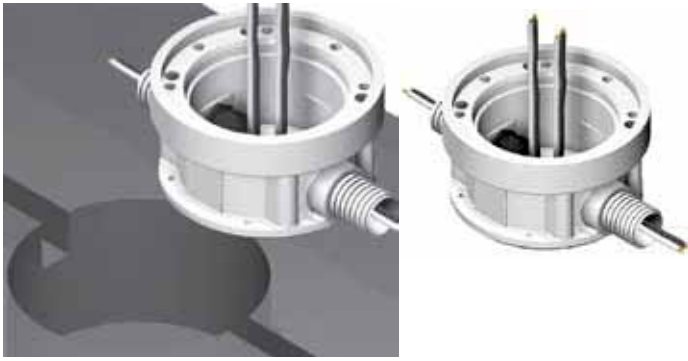
Boring core holes in the road surface / cable conduit
